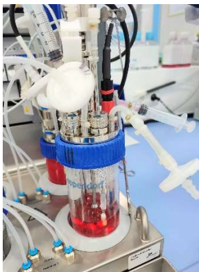
Figure 2: Stirred tank bioreactors used for process development (Eppendorf DASbox)
